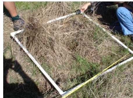
Quadrat used for randomly sampling vegetation within a predetermined area made of PVP pipe. This is a quick (and cheap) way to make 1 sq. ft. sized squares you can throw into a field as a marker. Photo: University of Idaho.
